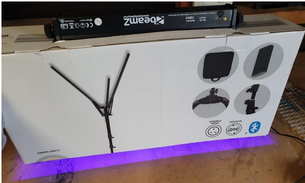
Fig 23: 405nm UV curing chamber
