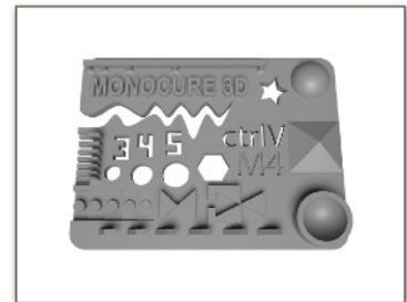
**8. Positioning it on the build plate** - Hopefully, you have followed my advice and downloaded the Mono Matrix from our website. It's time to open up your slicing software and position it on the build plate. Put it flat in the middle of the plate, with no supports or rafts. At this point, it might be necessary to slice the model (this is where the computer will figure out the slices and prepare them for the printer.) Now export the file in the format recommended by the printer manufacturer.
